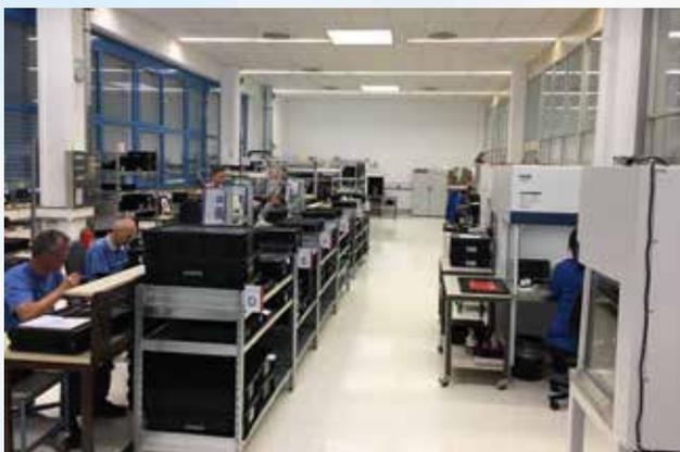
One of the most important markets for Hittech Prontor is the mechanical assembly of optical modules. Optical components (lenses, prisms, etc.) with a worth of more than three million Euro's are glued and assembled each year.
